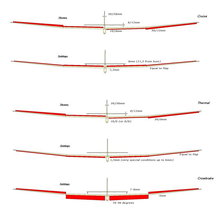
There is no elevator to flap mix (snap-flap) or Aileron to Rudder mix other than (although many pilots may use it):
